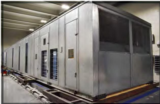
Customer Equipment in NAIC Sound Test Chamber
